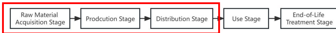
Figure 2: System Boundary (The red box represents the system boundary for the product life cycle in this report)
